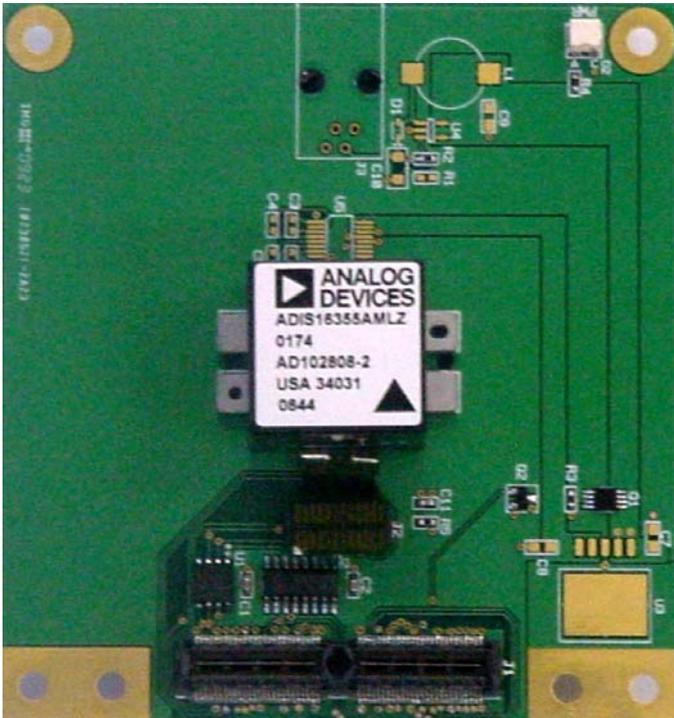
This sensor provides Roll, Pitch and Yaw rate (up to 300 degrees per second) and linear acceleration. It has on board monitors for power supply and gyro temperatures.
